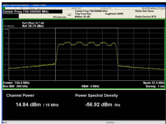
Figure 31: 16QAM 15MHz B.W.; 750.5MHz, 30kHz
