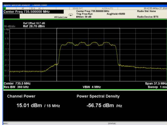
Figure 26: 16QAM 15MHz C.S; 735.5MHz, 60kHz
