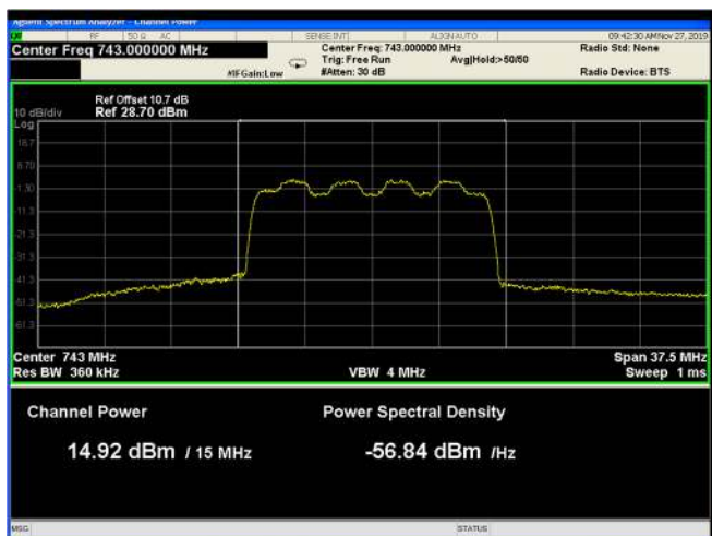
Figure 29: 16QAM 15MHz B.W.; 743.0MHz, 60kHz
