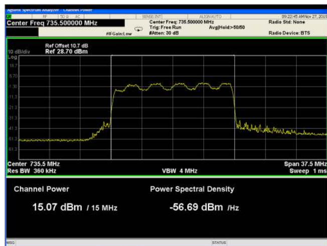
Figure 24: 16QAM 15MHz B.W.; 735.5MHz, 15kHz
