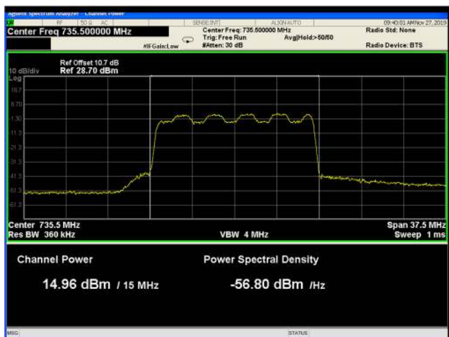
Figure 25: 16QAM 15MHz B.W.; 735.5MHz, 30kHz
