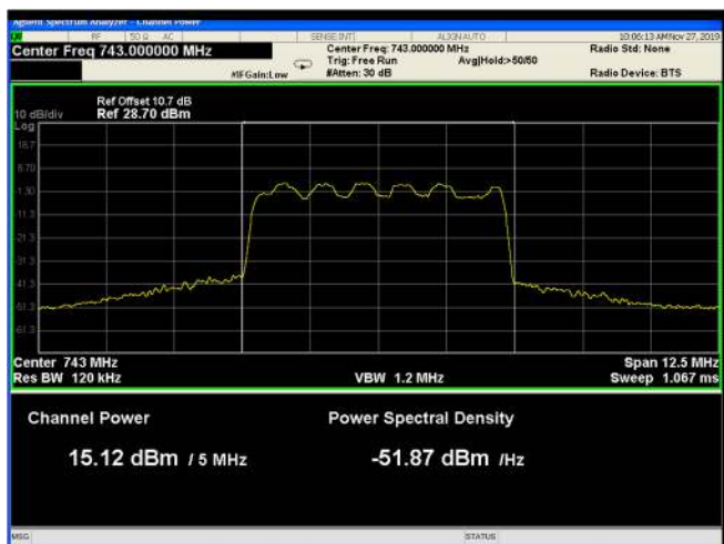
Figure 11: 16QAM 5MHz B.W.; 743.0MHz, 15kHz
