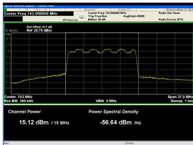
Figure 28: 16QAM 15MHz B.W.; 743.0MHz, 30 kHz
