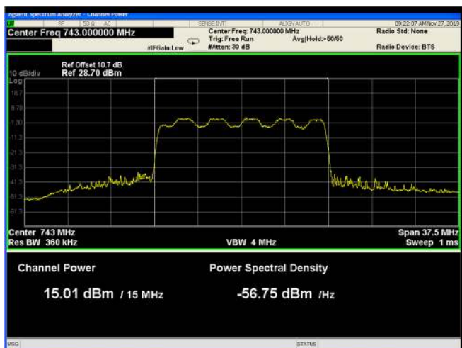
Figure 27: 16QAM 15MHz B.W.; 743.0MHz, 15kHz
