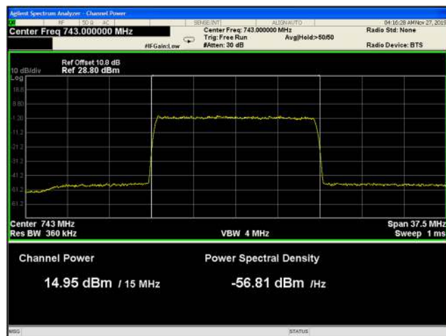
Figure 60: 64QAM 15MHz B.W.; 743.0MHz, 15kHz
