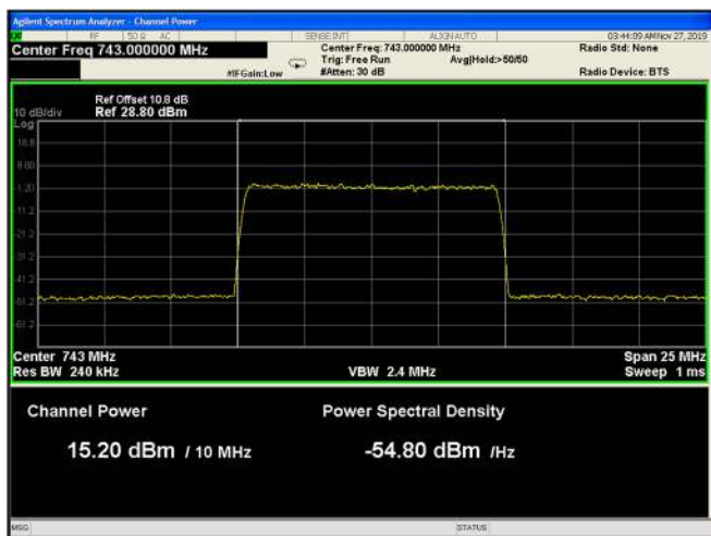
Figure 51: 64QAM 10MHz B.W.; 743.0MHz, 15kHz
