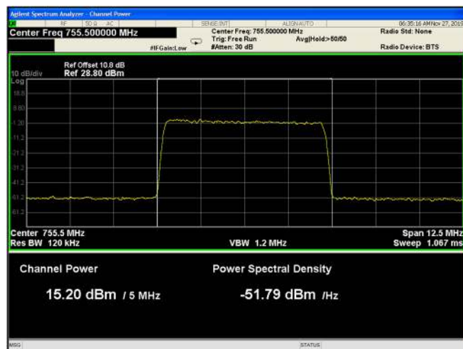
Figure 46: 64QAM 5MHz B.W.; 755.5MHz, 15kHz
