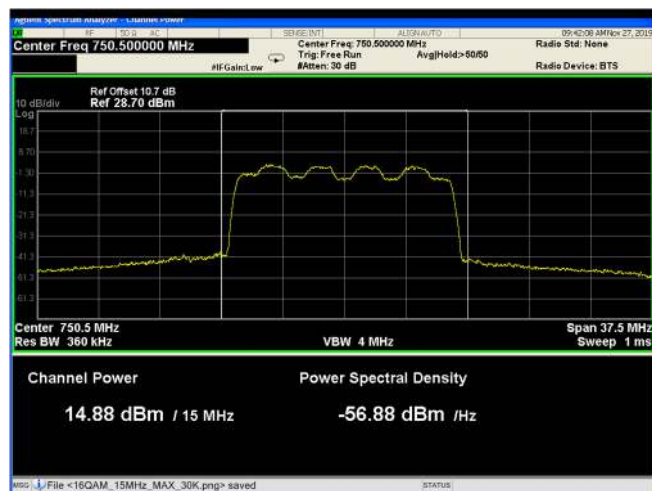
Figure 32: 16QAM 15MHz B.W.; 750.5MHz, 60kHz
