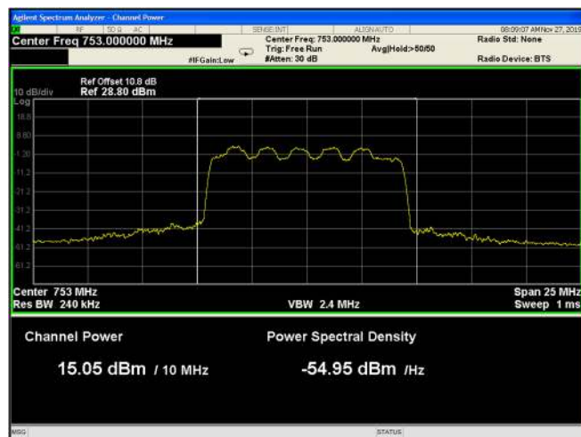
Figure 22: 16QAM 10MHz C.S; 753.0MHz, 30kHz
