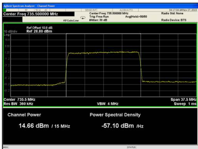
Figure 57: 64QAM 15MHz B.W.; 735.5MHz, 15kHz
