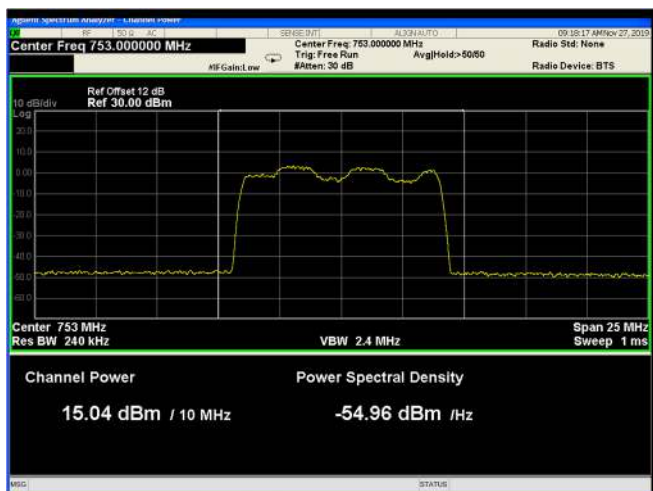
Figure 23: 16QAM 10MHz B.W.; 753.0MHz, 60kHz
