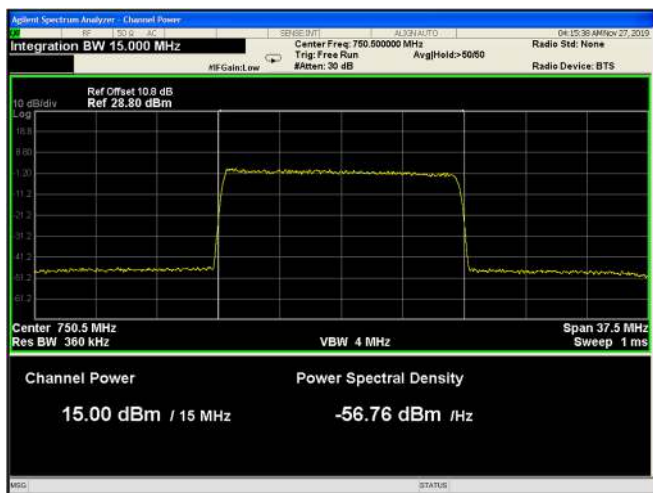
Figure 63: 64QAM 15MHz B.W.; 750.5MHz, 15kHz
