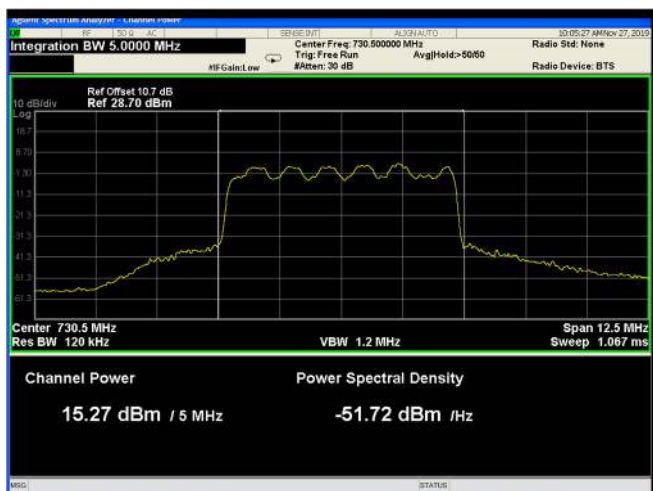
Figure 9: 16QAM 5MHz B.W.; 730.5MHz, 15kHz
