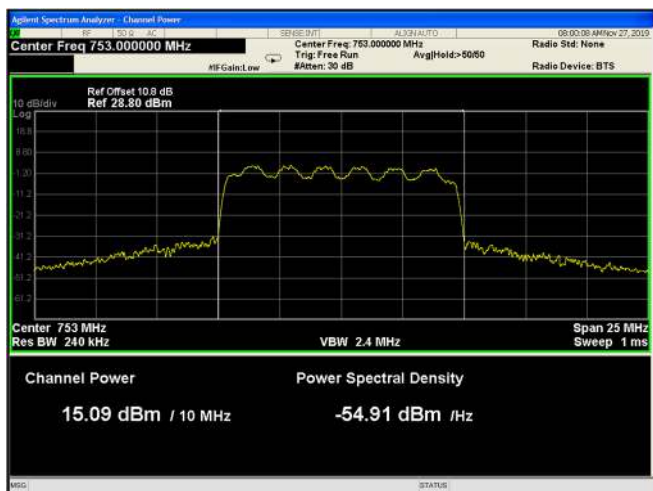
Figure 21: 16QAM 10MHz B.W.; 753.0MHz, 15kHz
