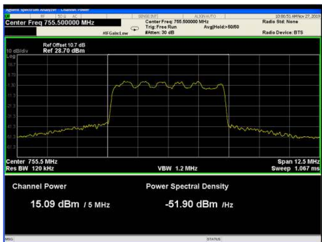
Figure 13: 16QAM 5MHz B.W.; 755.5MHz, 15kHz
