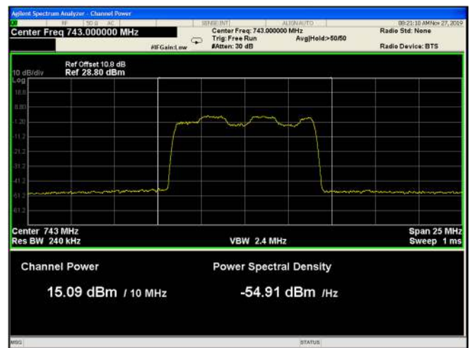
Figure 20: 16QAM 10MHz B.W.; 743.0MHz, 60kHz
