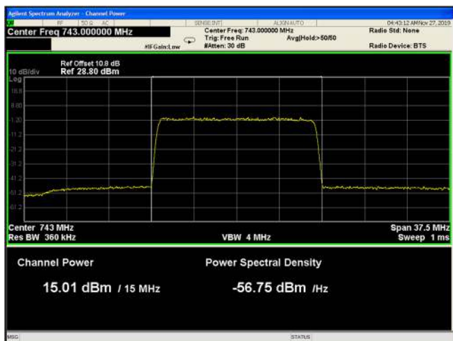
Figure 61: 64QAM 15MHz; 743.0MHz B.W., 30kHz
