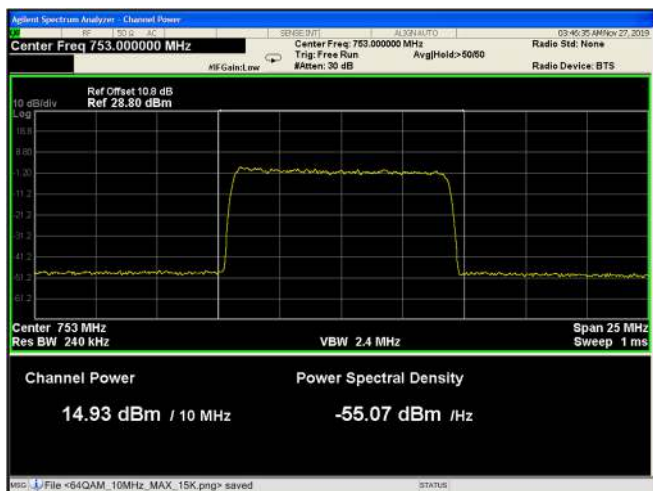
Figure 55: 64QAM 10MHz B.W.; 753.0MHz, 30kHz
