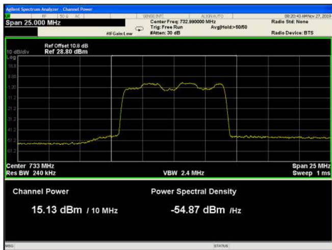
Figure 17: 16QAM 10MHz B.W.; 733.0(732.9) MHz, 60kHz
