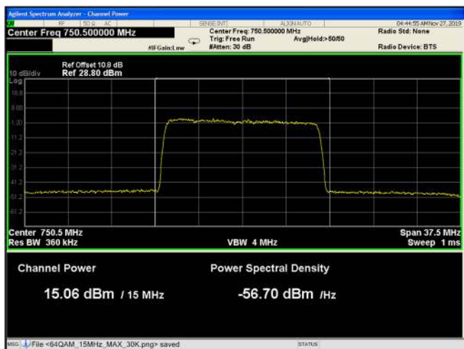
Figure 65: 64QAM 15MHz B.W.; 750.5MHz, 60kHz
