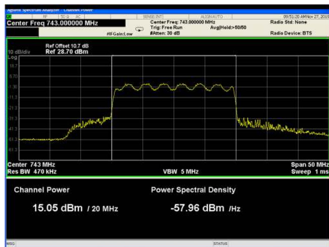
Figure 36: 16QAM 20MHz B.W.; 743.0MHz, 15kHz
