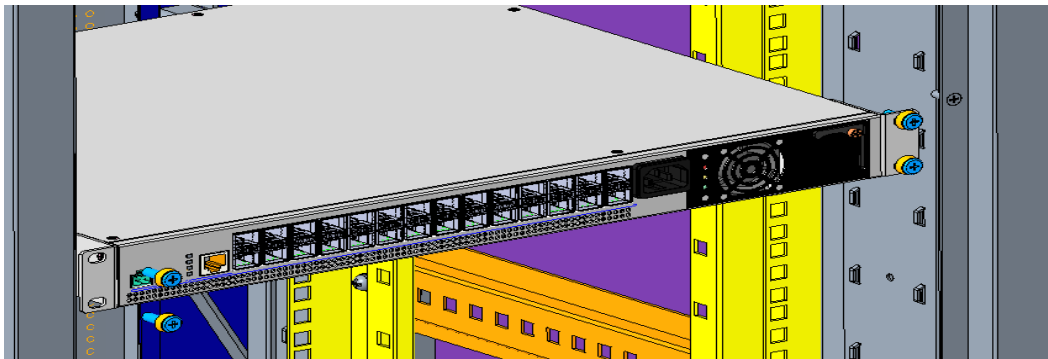
Figure 37. Rack Installation - Step 2
