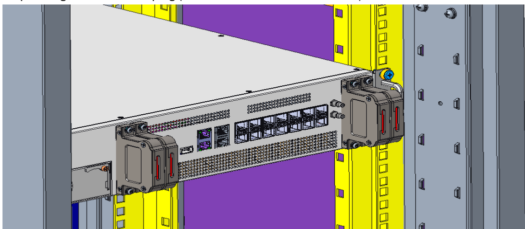
Figure 34. DCU RF Cable Plug Installation
