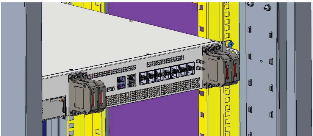
Figure 30. DCU RF Cable Plug Installation
