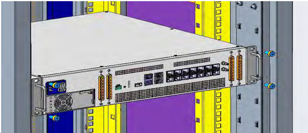
Figure 30 Installation diagram of DCU in the Rack
