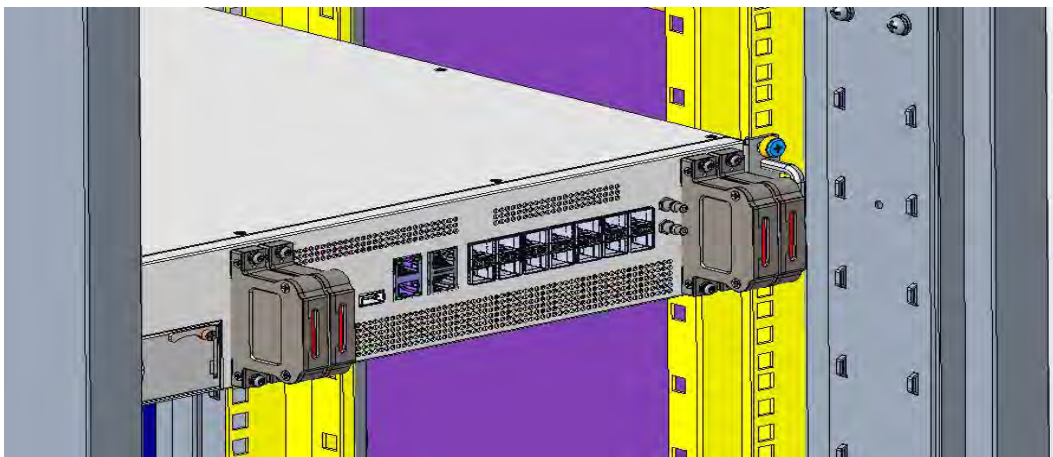
Figure 31 DCU RF cable plug installation
