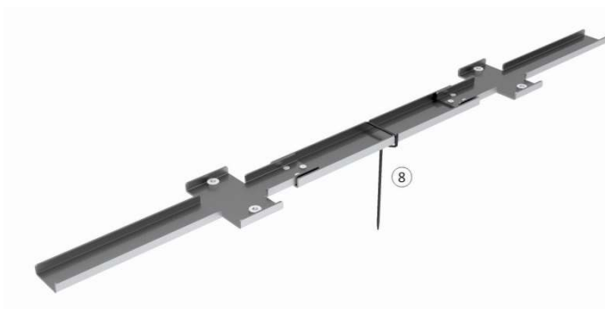
Figure 62. Attaching Cable Tie to Mounting Bracket
