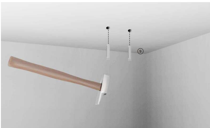
Figure 50. Insert Plastic Wall Plugs
