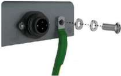
Figure 29. Connect Ground Cable at Rear Side
