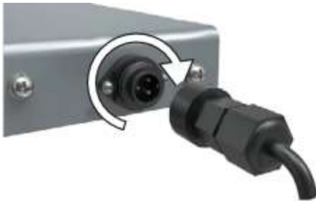
Figure 15. Connect Power Cable at Rear Side
