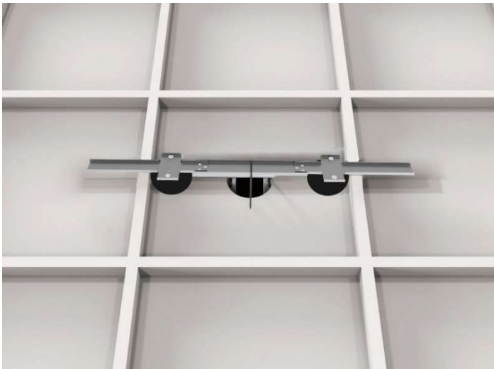
Figure 65. Placing the Bracket I & VI 2
