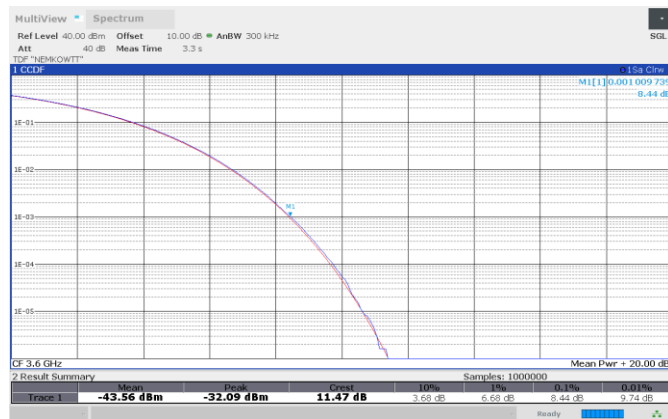
Figure 8.4-5: 0.1% PAPR results, narrowband signal, 0.5 dB below and 3 dB above AGC threshold
