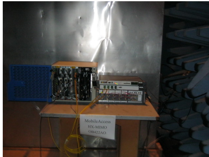
Figure 2. Conducted Emission From AC Mains Test
