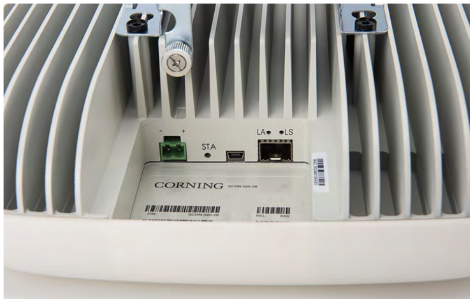
Figure 4 SCRN-520 Connectors and Status LED
