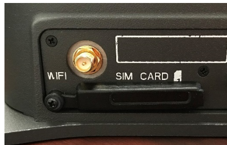
Figure 2-8 Secure the SIM Card Cover
