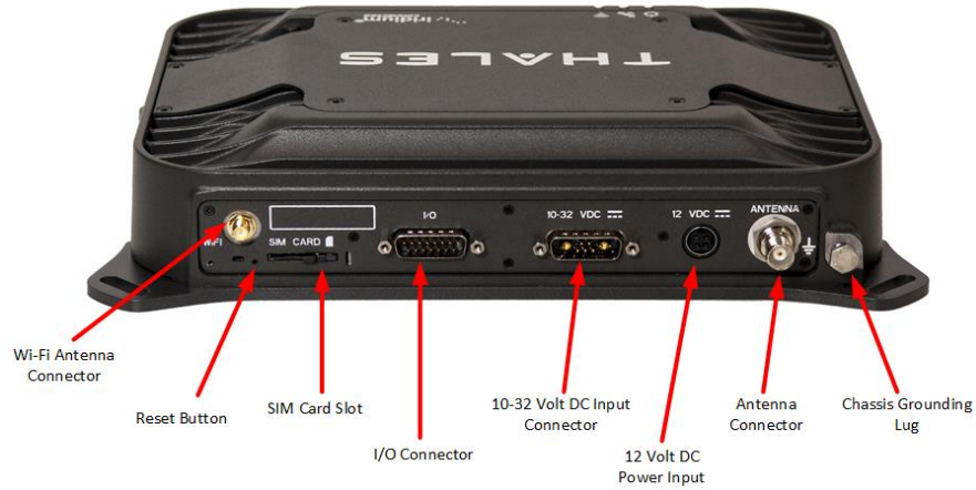
Figure 1-5 Terminal Unit (TU) Back Panel Detail
