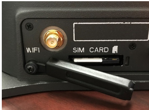
Figure 2-6 SIM Card with Cover Opened
