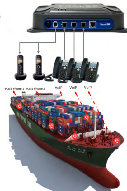
Figure 2-2 Local Communications via PBX Functionality
