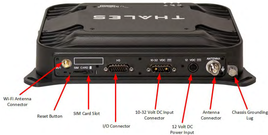
Figure 2-7 Below Deck Unit (BDU) Back Panel Detail
