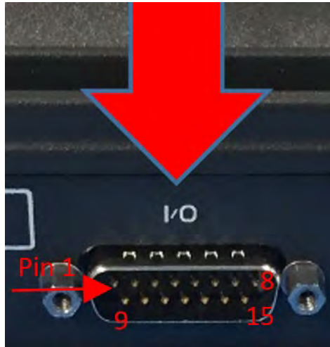
Figure 7-2 GPIO Connector Pin Detail
