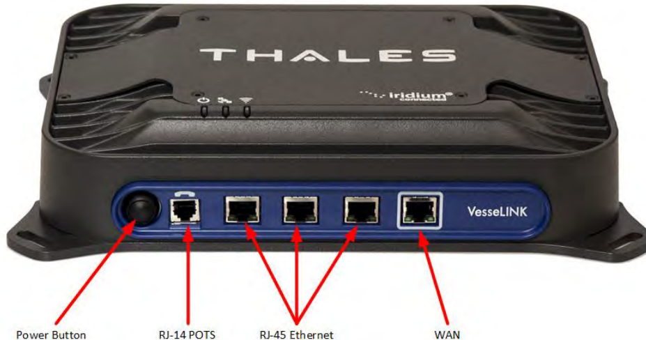
Figure 3-1 BDU Front Panel Detail
