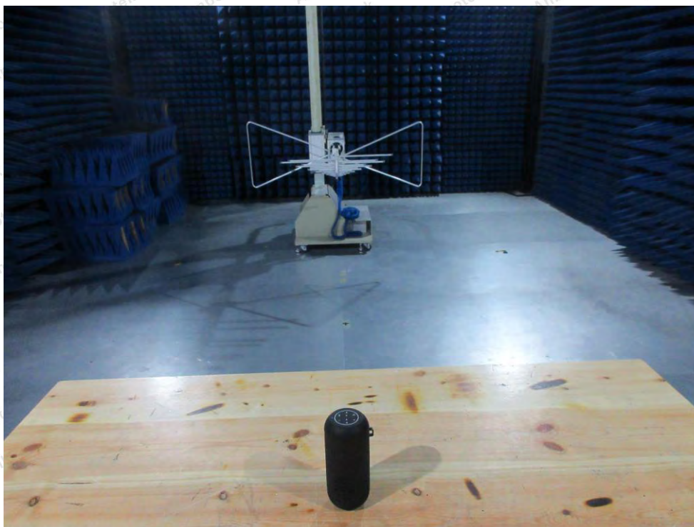
Photo of Radiation Emission Test
