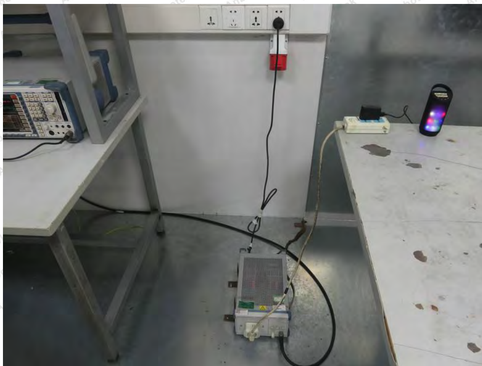
Photo of Conducted Emission Measurement
