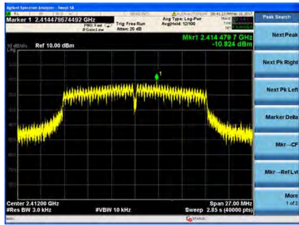
(802.11g) PSD plot on channel 6
