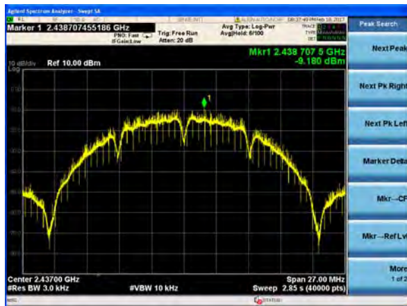
(802.11b) PSD plot on channel 11
