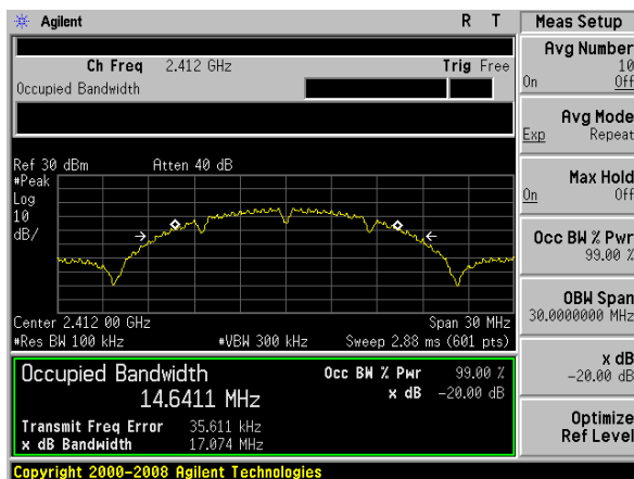
(802.11b) -20dB Bandwidth plot on channel 6
