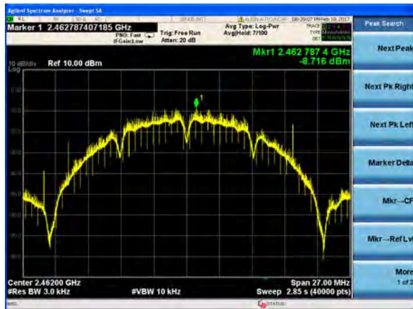
(802.11b) PSD plot on channel 11
