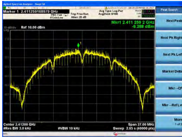
(802.11b) PSD plot on channel 6
