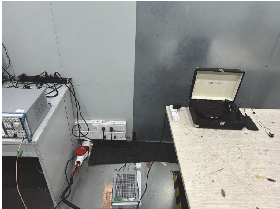
Conducted Emission Test Setup
