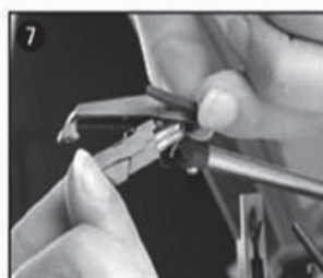
separate the cartridge from the socket lightly.
