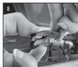
take off the audio-line from the cartridges completely.
