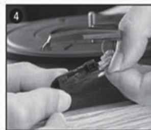
take off the audio-line from the cartridges completely.
