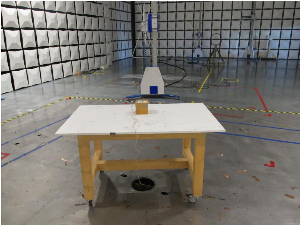
Figure 12 - Test setup for radiated emission
