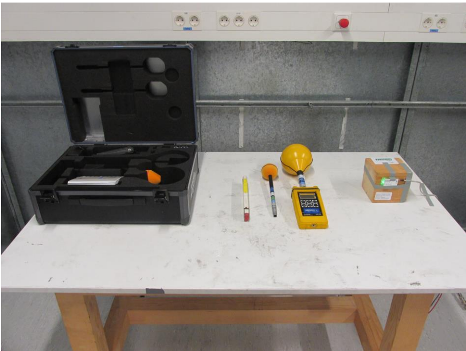
Figure 15 - Test setup for Exposure of Humans to RF Fields
