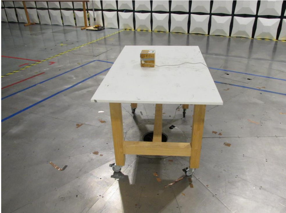
Figure 13 - Test setup for radiated emission
