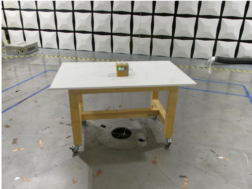
Figure 10 - Test setup for radiated emission
