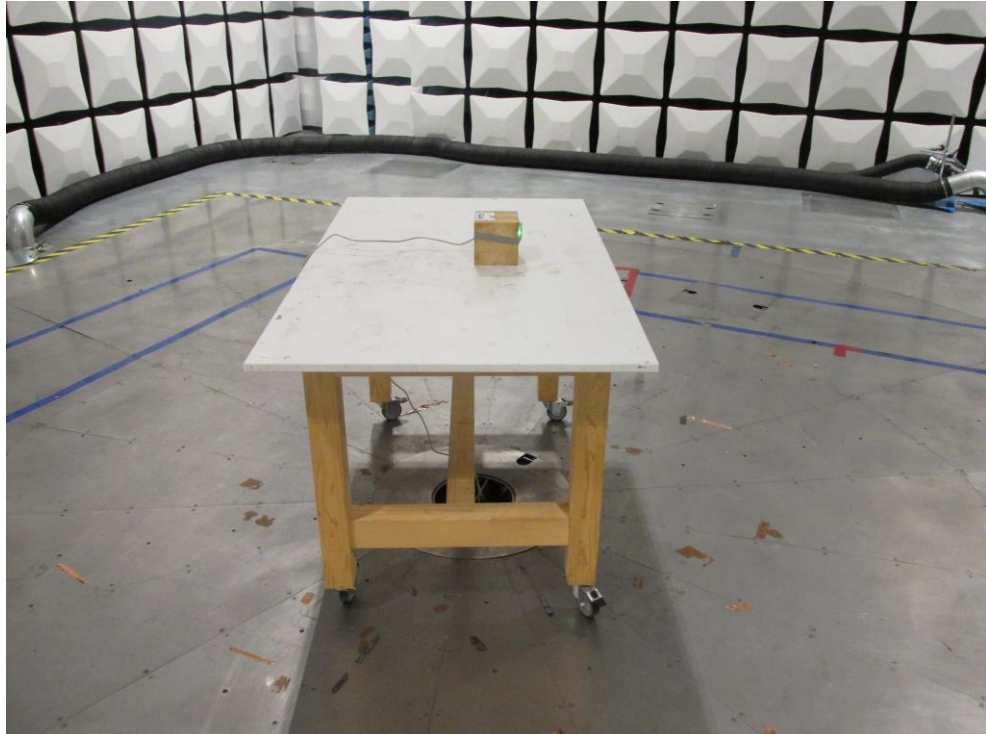
Figure 11 - Test setup for radiated emission
