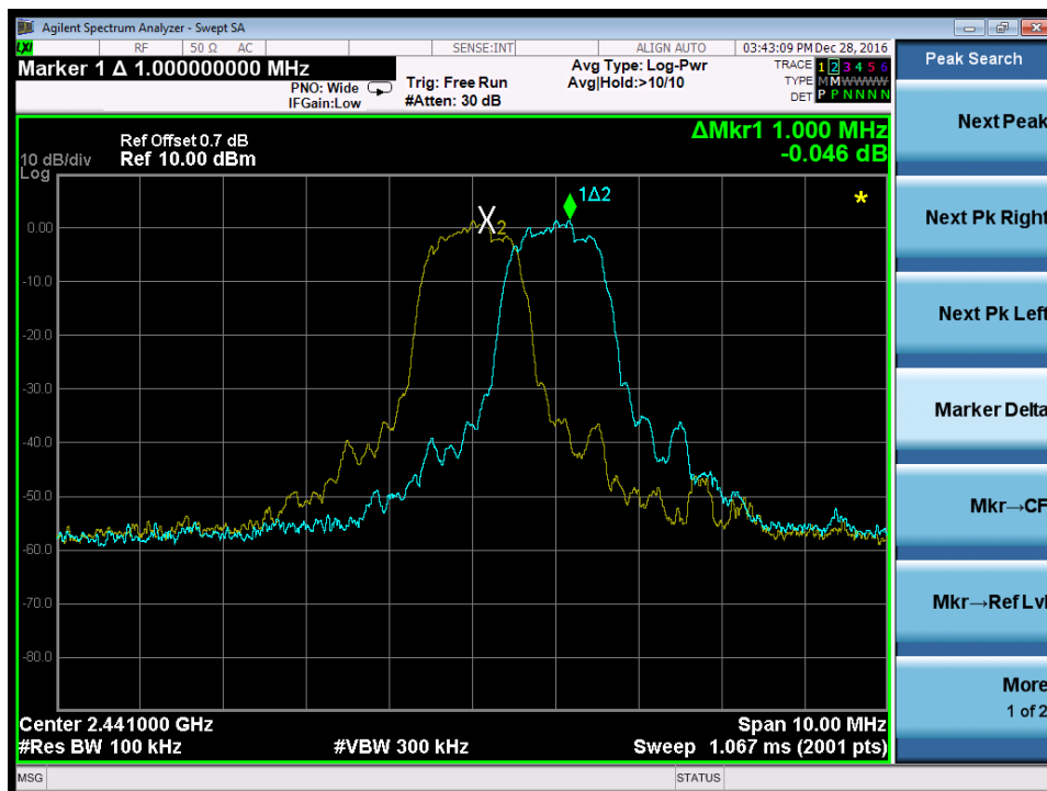
Figure 32: Frequency Separation, TM12, observation Frequency 2441MHz
