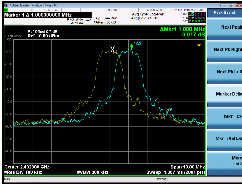
Figure 31: Frequency Separation, TM12, observation Frequency 2402MHz
