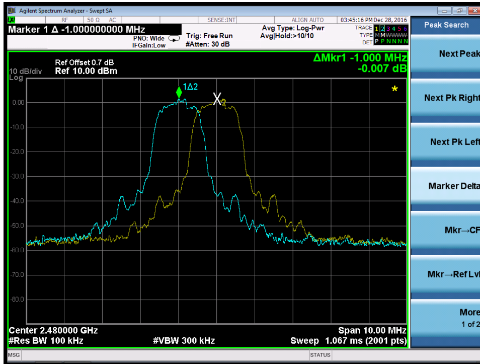
Figure 33: Frequency Separation, TM12, observation Frequency 2480MHz
