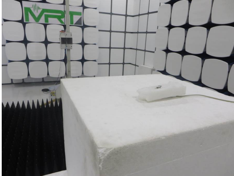
Photograph 3: Set-up for Radiated Test above 1GHz
