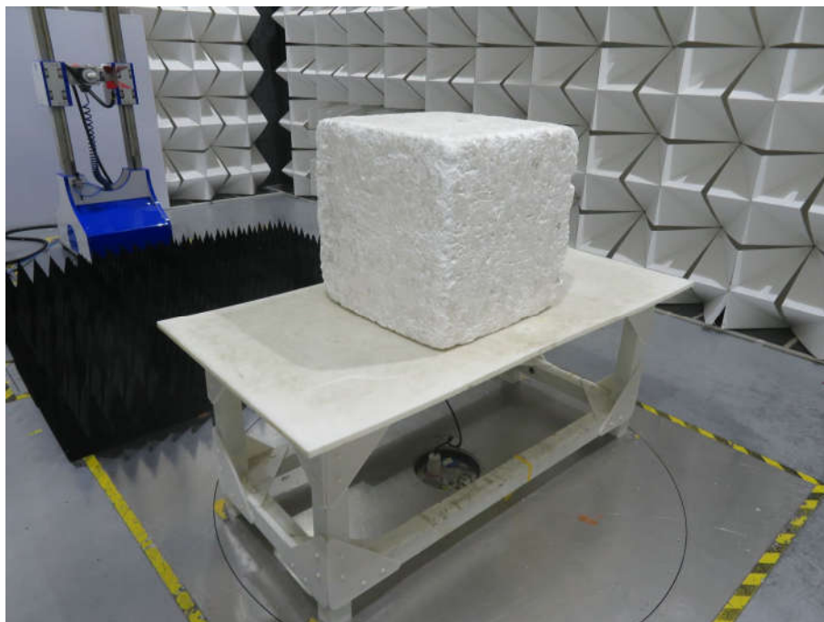
Radiated spurious emission Test Setup-3(Above 1GHz)
