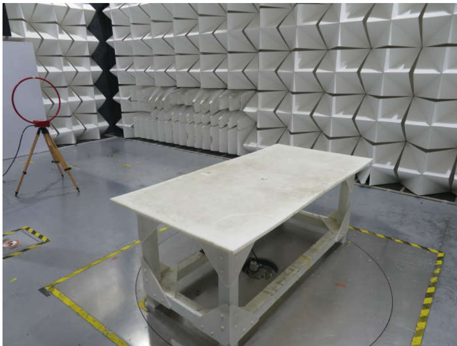
Radiated spurious emission Test Setup-1(9kHz-30MHz)
