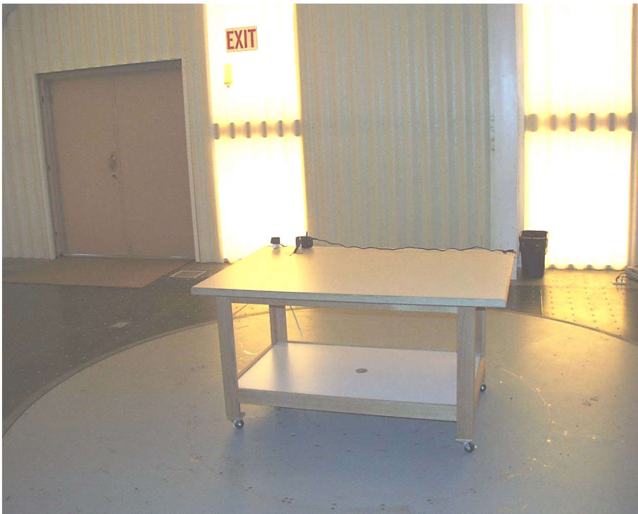
Front View Radiated Emission Configuration (Horizontal Orientation)
