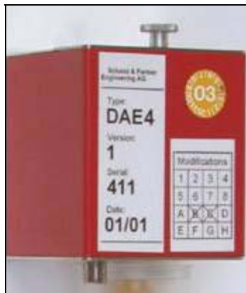
Figure 9: Data acquisition electronics
