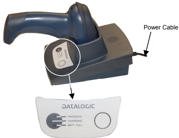
Figure 1 – OM-1000 BT Charging Batteries
