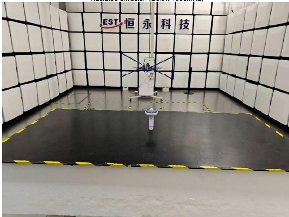
Radiated emission (Above 1000MHz)
