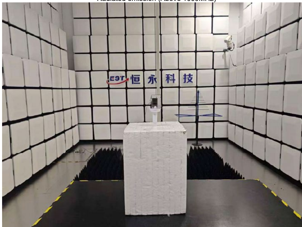
Radiated emission (Above 1000MHz)
