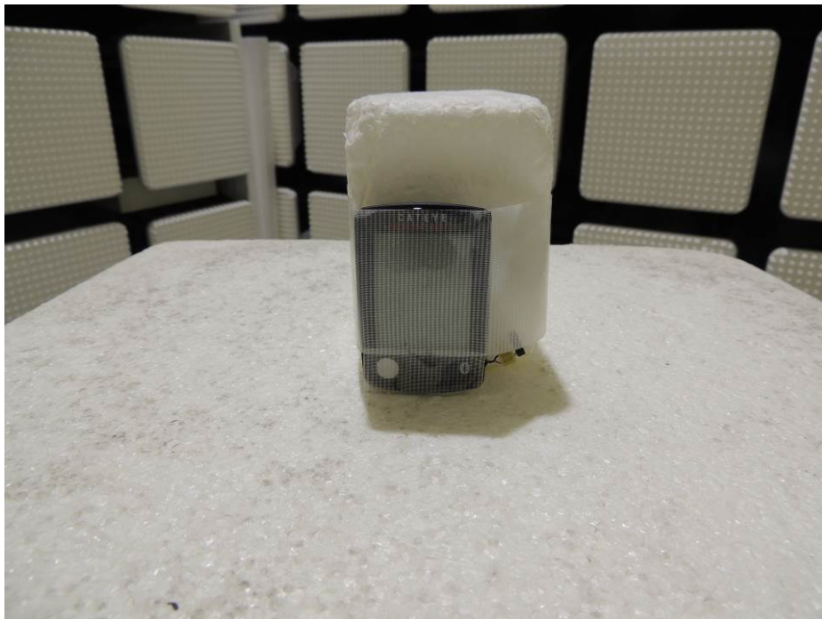
Photograph 5: Set-up for Radiated Emission, EUT Configuration Y-Axis
