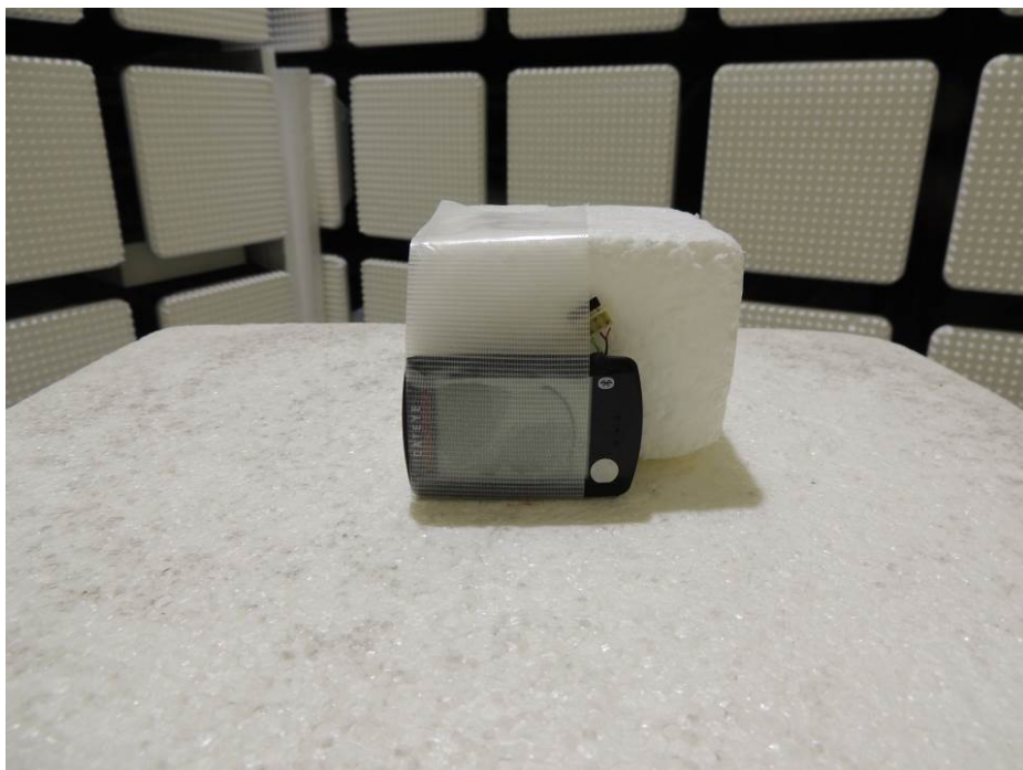
Photograph 6: Set-up for Radiated Emission, EUT Configuration Z-Axis
