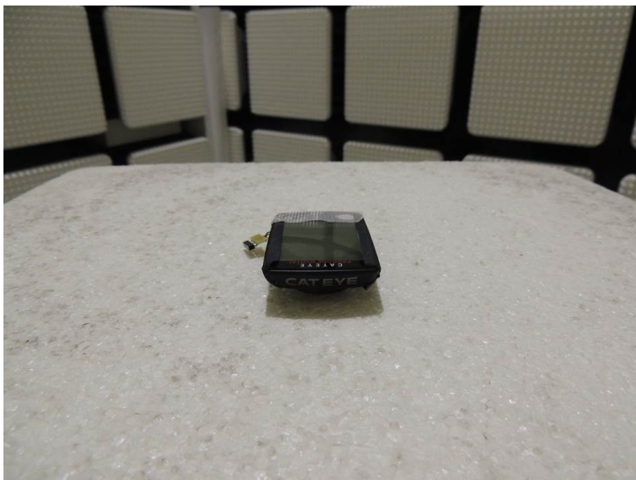
Photograph 4: Set-up for Radiated Emission, EUT Configuration X-Axis
