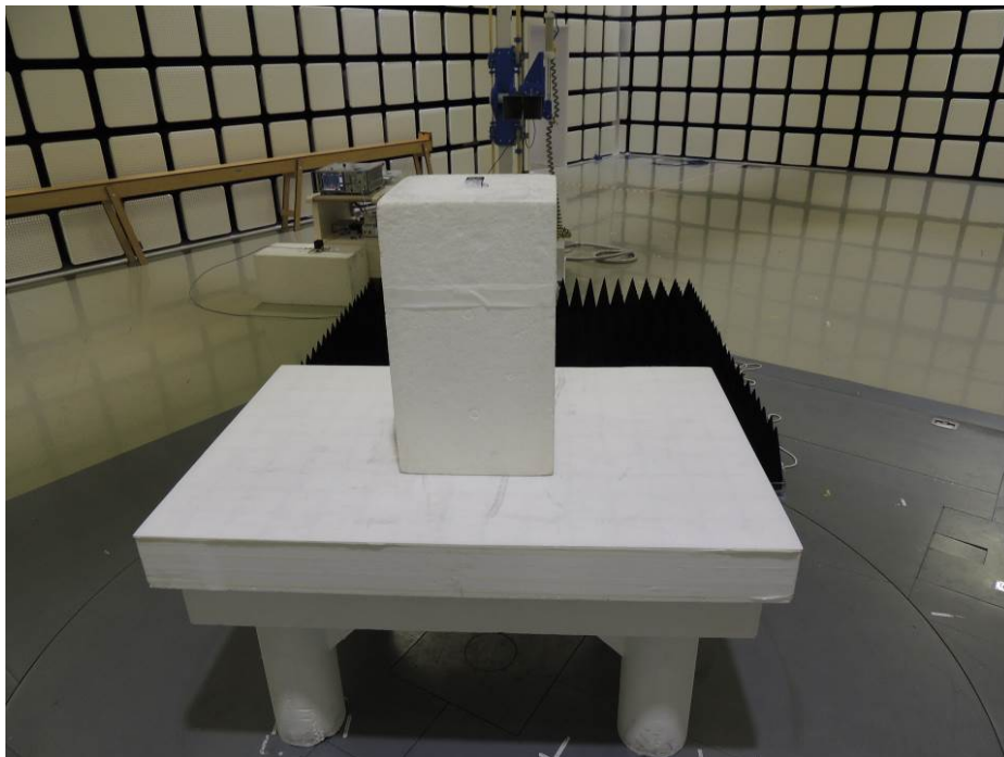
Photograph 3: Set-up for Radiated Emission of Transmitter, Rear View
