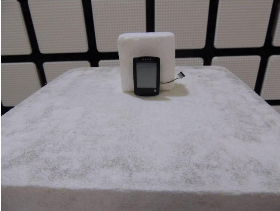
Photograph 8: Set-up for Radiated Emission, EUT Configuration Y-Axis at 1.5m height
