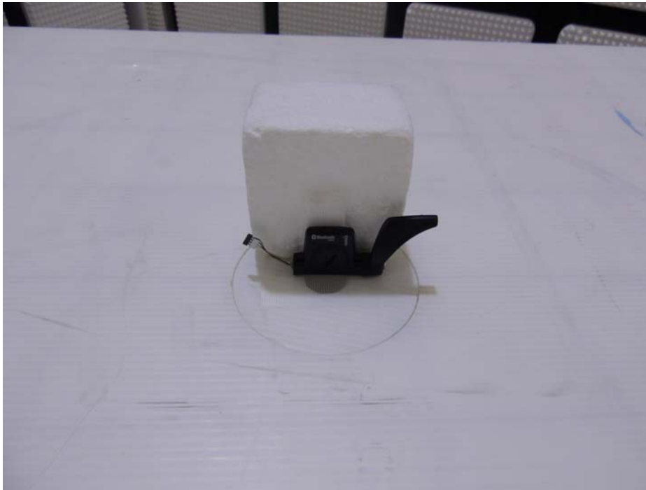
Photograph 6: Set-up for Radiated Emission, EUT Configuration Y-Axis
