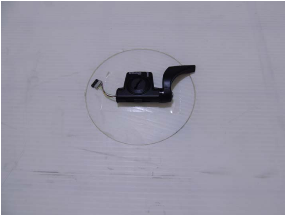
Photograph 5: Set-up for Radiated Emission, EUT Configuration X-Axis
