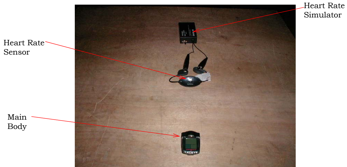
Main Body and Heart Rate Sensor
