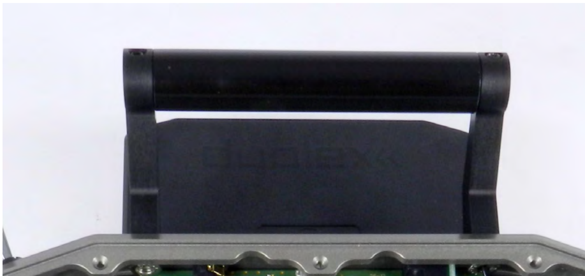
Figure 2b – Antenna 900MHz
