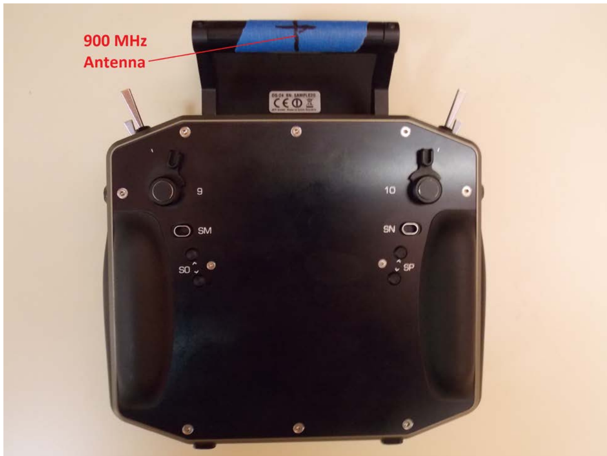
Back of Device and 900 MHz Antenna Location
