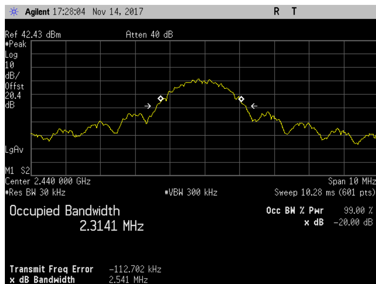
Figure 7.3.4.2-8: 20 dB BW – Middle Channel (AP2)
