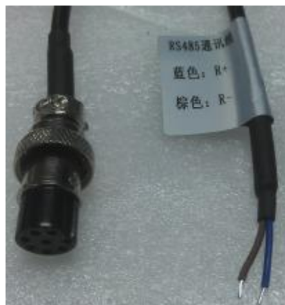
Pic 6 RS485config cable
