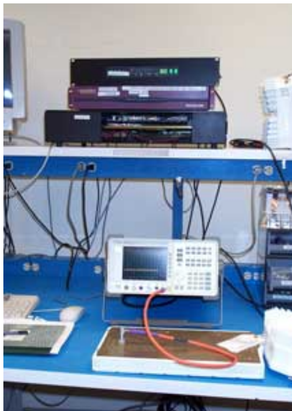
Figure 2 Base Station ODU 9kHz-40GHz Test Set Up
