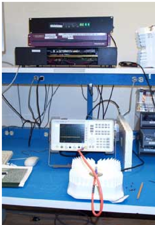
Figure 5 CPE ODU 9 kHz-200 GHz Test Set Up
