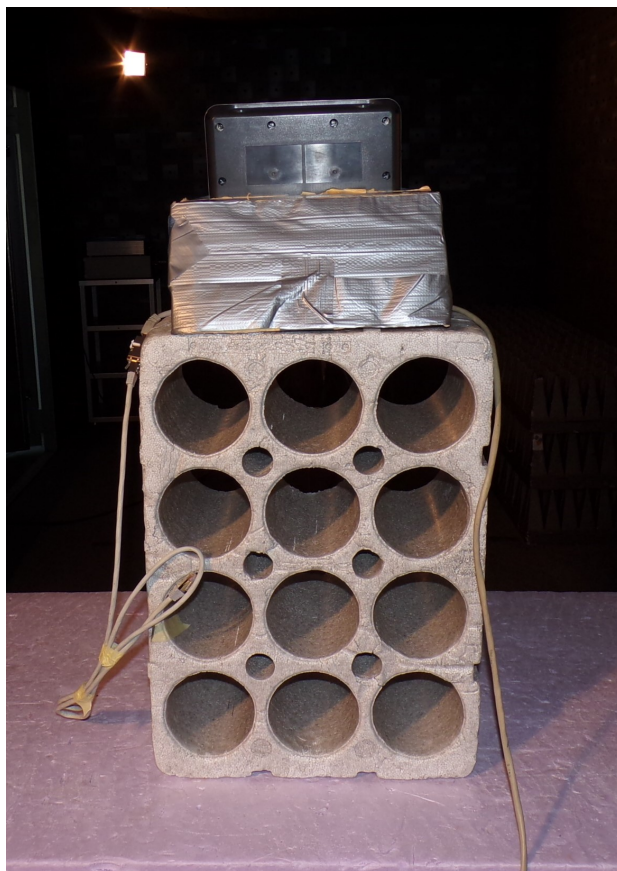
Full Anechoic chamber (Freq > 1GHz)
