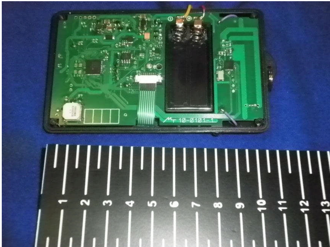
Photograph shows the main circuit board. The 915MHz antenna element is shown etched into the printed circuit board (right-hand side)
