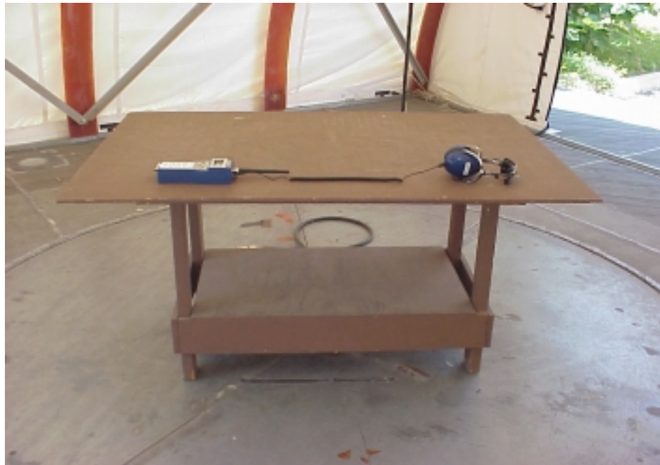
5.1 Photo: Radiated Emissions (Front View)
