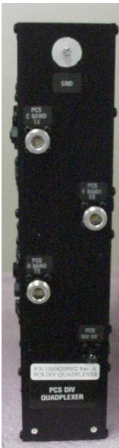
Figure 6-5 Quadplexer, PCS Diversity (Transmitting Blocks C/D/E)
