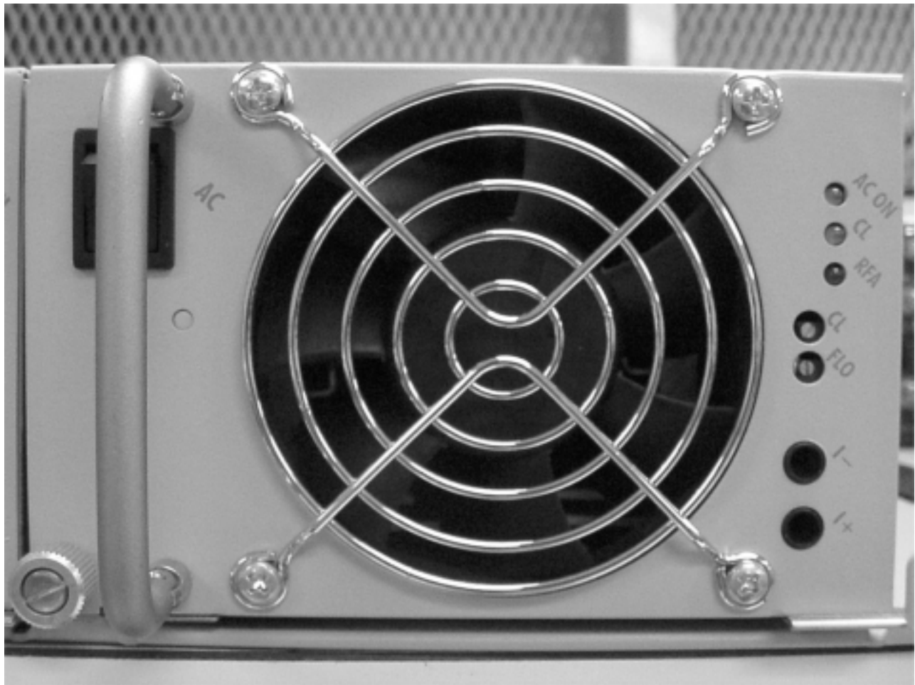
Figure 13. RAN Rectifier Front Panel
