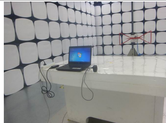
Conducted Emissions Test Setup Front View
