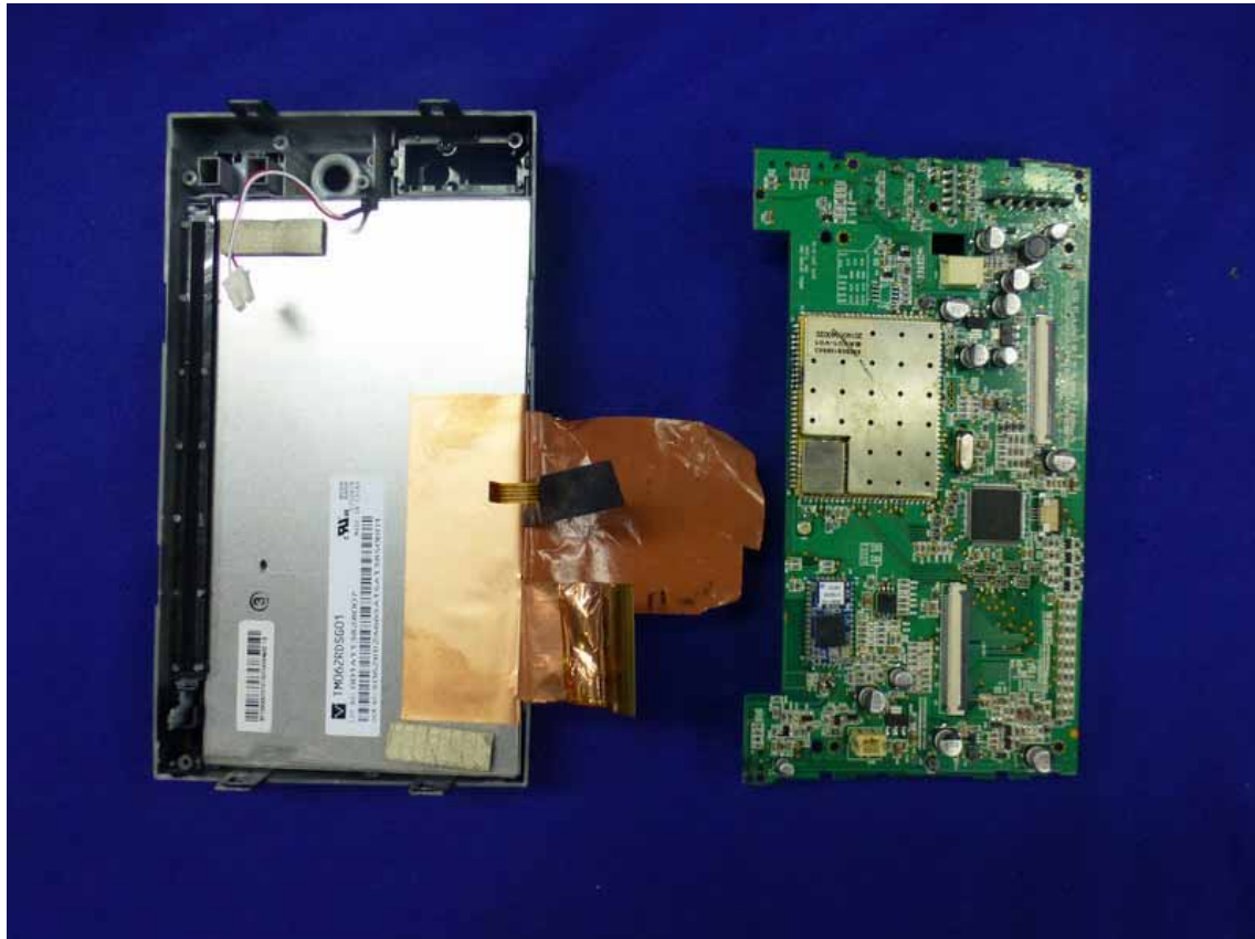
Figure 28 General Inside of the EUT
