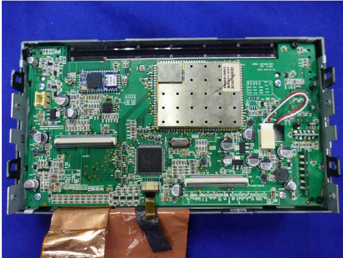
Figure 28 General Inside of the EUT
