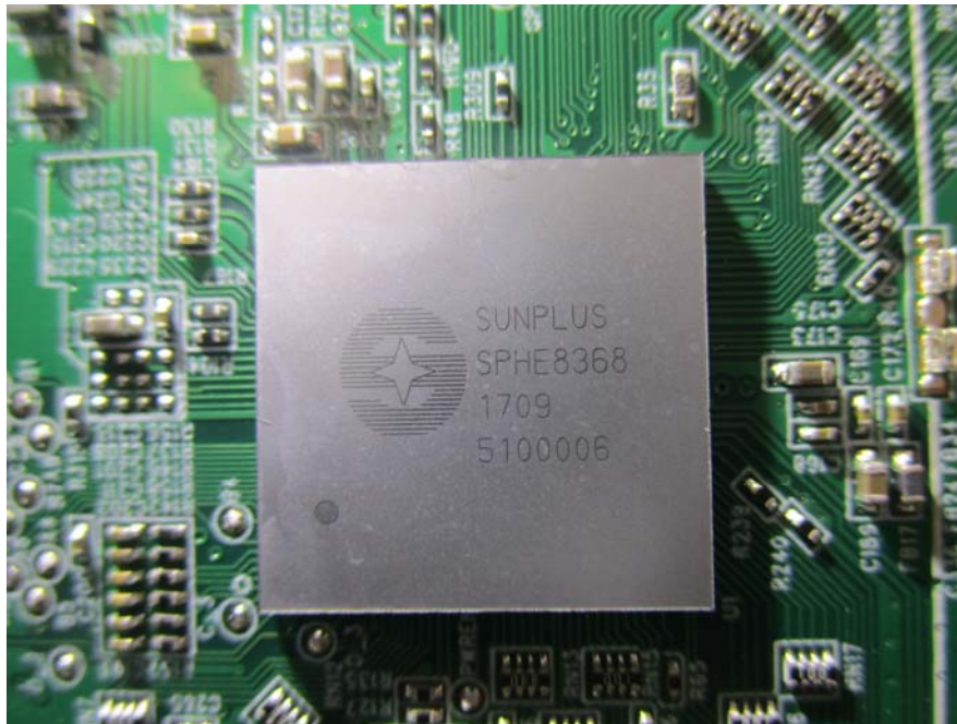
EUT – Main Chip View
