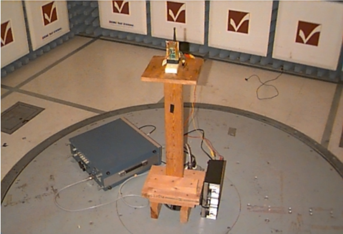
View of the K & A Wireless model VTRAN-2500 module during the Radiated Emissions tests. This view shows the orientation of the product during tests of the emission from the system.
