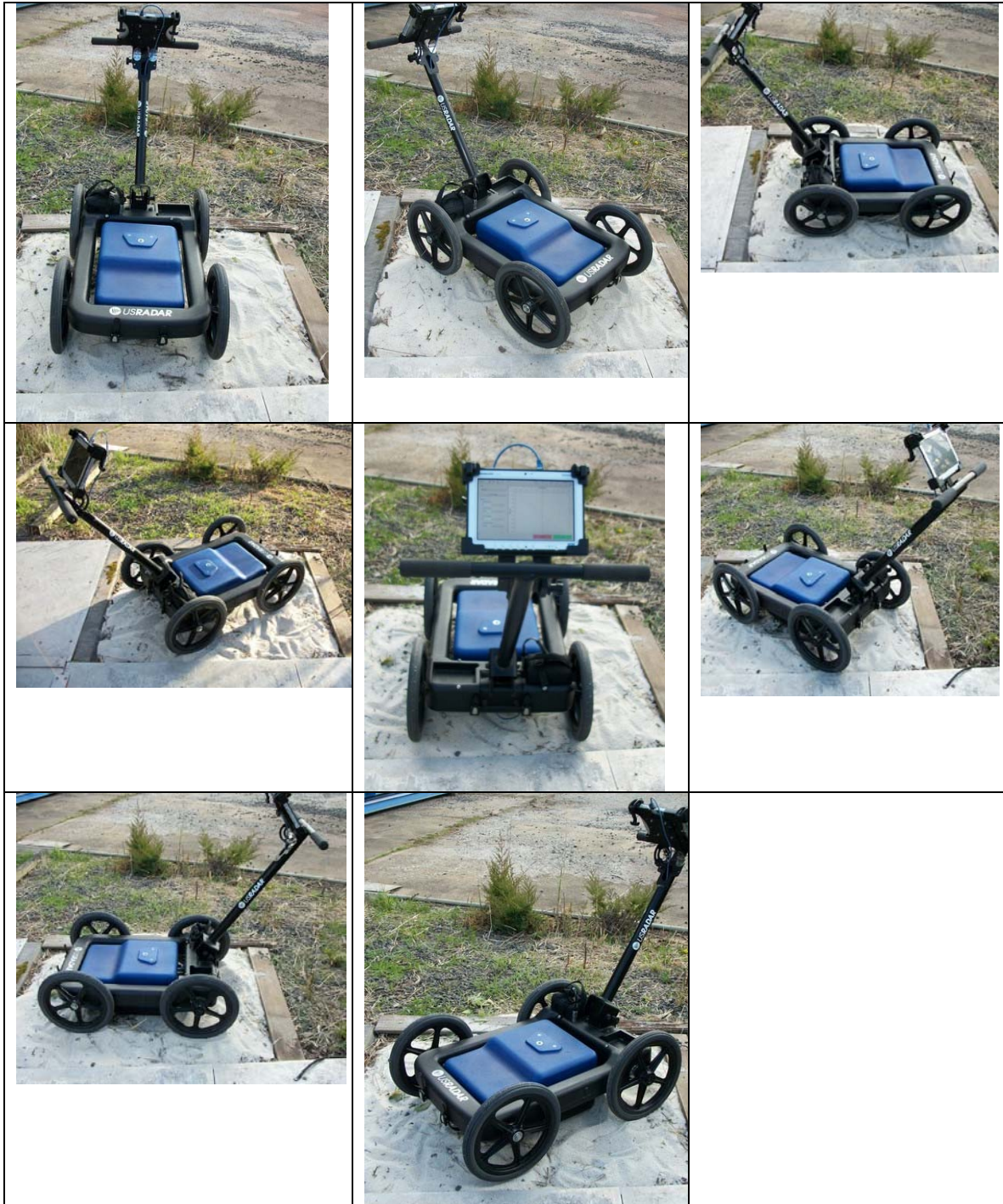
EUT Positions with 45 Degree Interval
