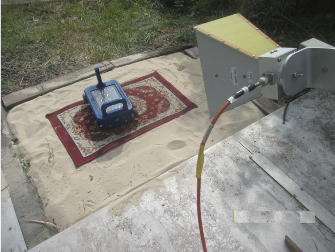
Above 1GHz ( 1m measurement for low emission signals)
