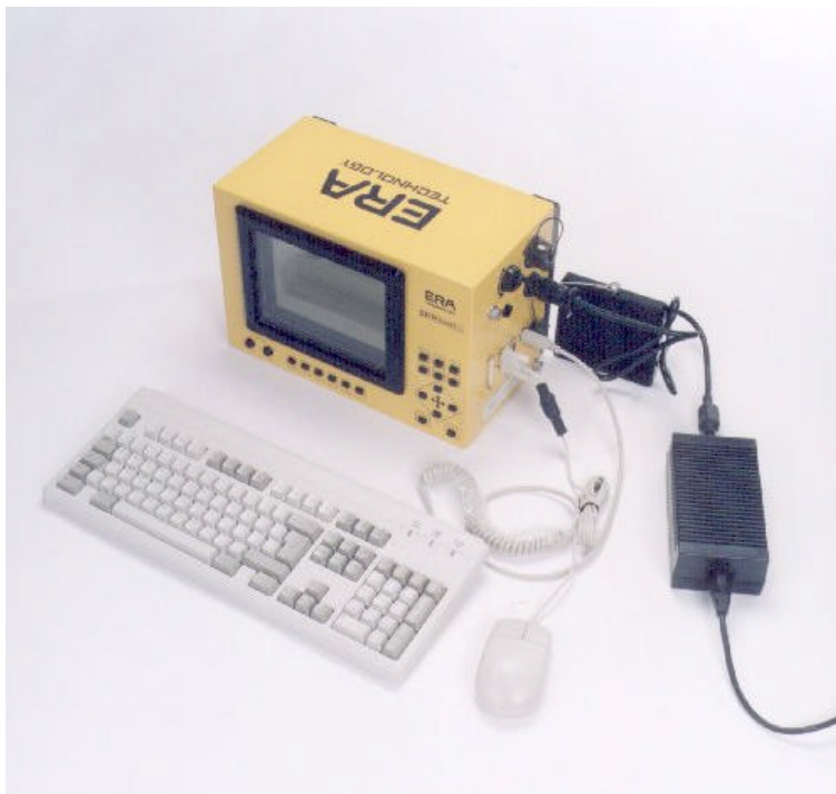
Figure 2 SPRscan controller in office mode
