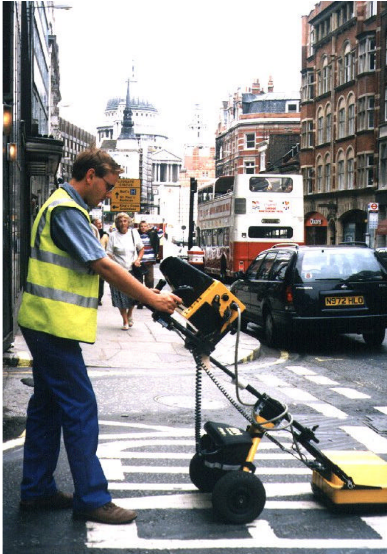
Figure 3 SPRscan with 500MHz antenna in use
