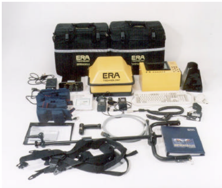
Figure 1 SPRscan system disassembled with 500MHz antenna
