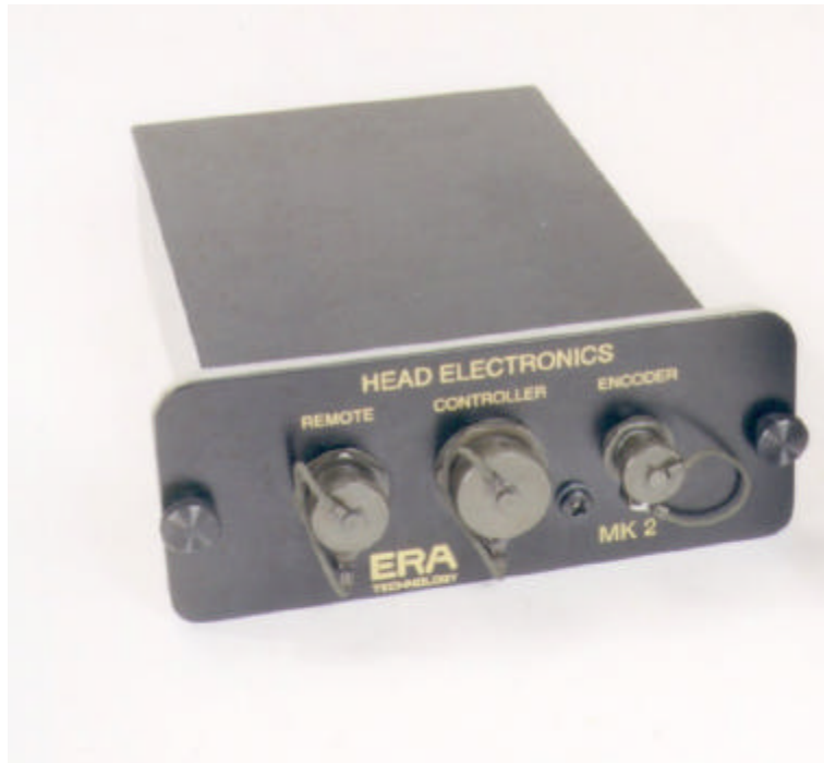
Figure 5 SPRscan head electronics
