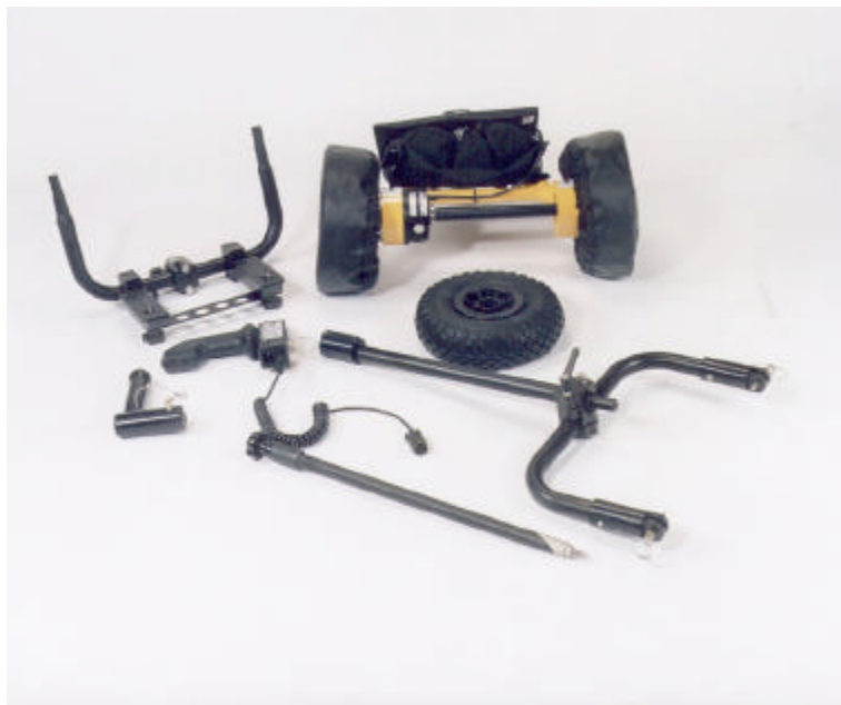
Figure 4 SPRscan trolley incorporating encoder
