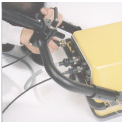
Connect the three cables to the Head Electronics unit in the antenna
