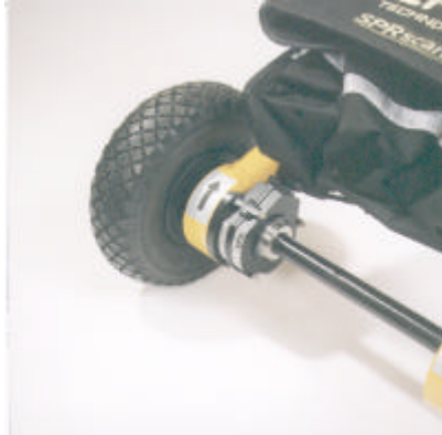
Position the trolley wheels so that the arrows point forward
