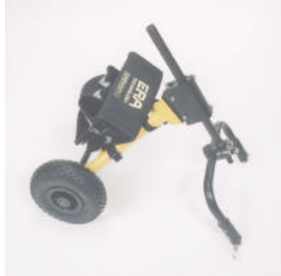
Fix the clevis and handle shaft to the wheels
