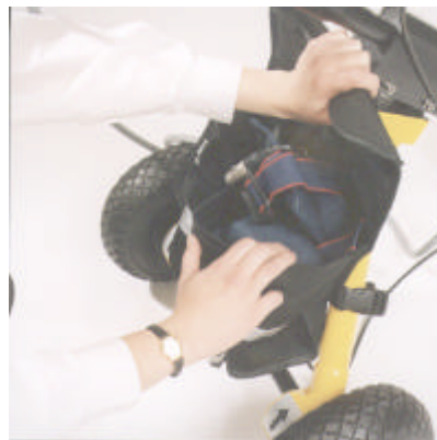
Place the batteries in the battery bag
