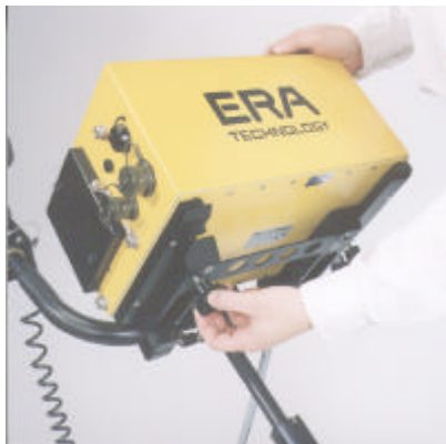
Fix the controller in place with the two screws
