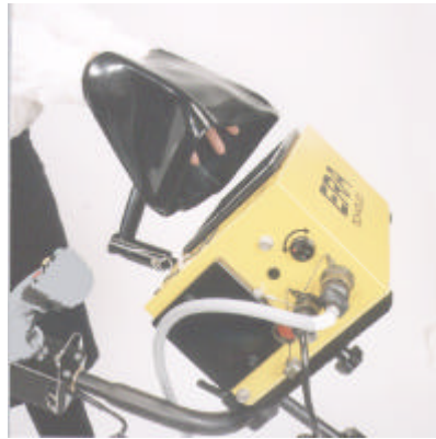
Fix the visor on the controller
