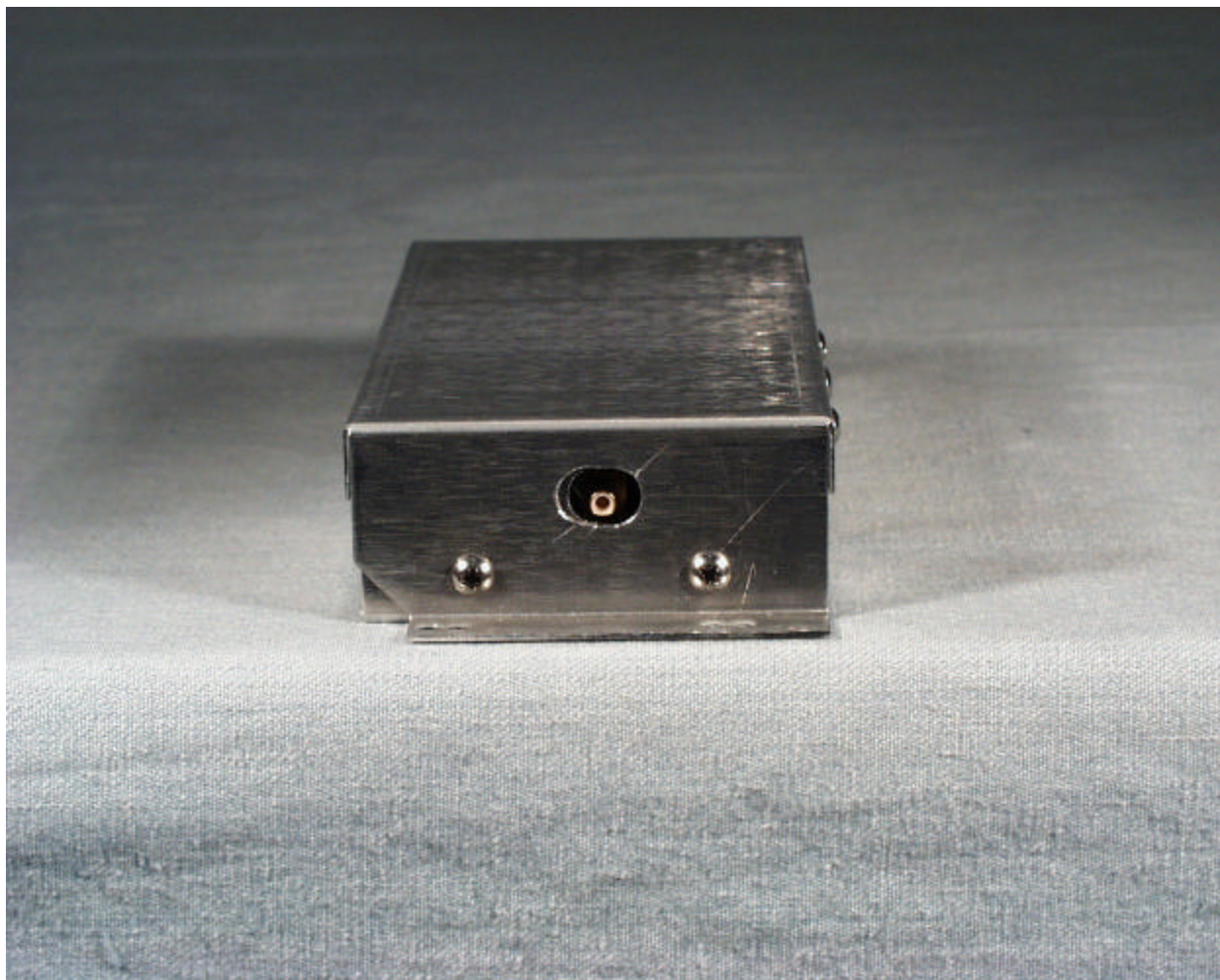
End View of the 2MOD-6322-A411 showing the antenna connector
