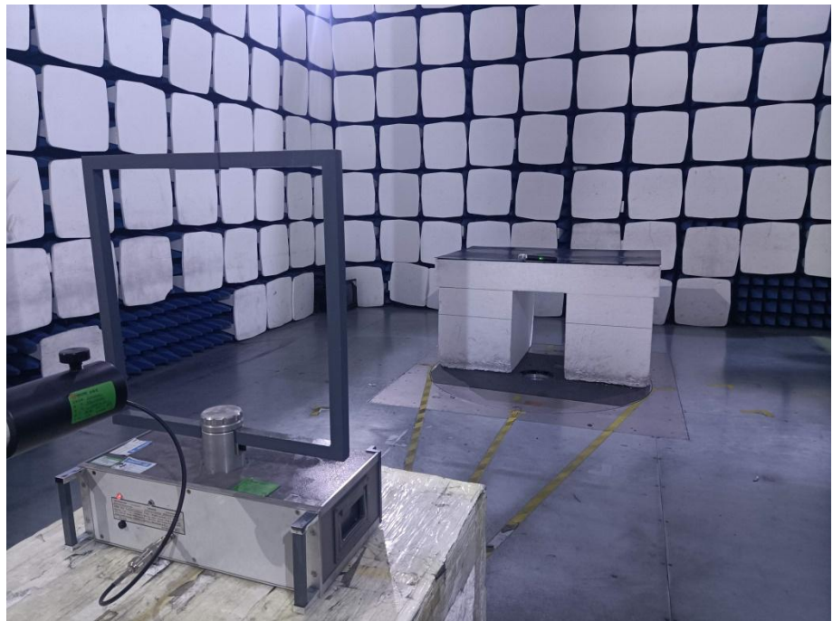
Radiation Emission Test Setup (Below 30MHz)
