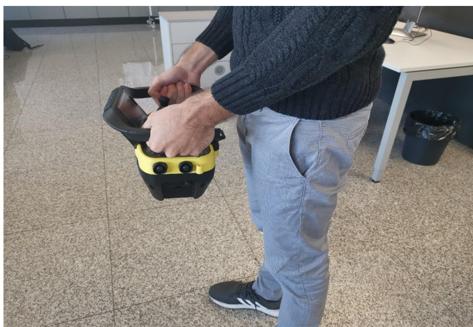
Figure F.7: Correct working position using PJM unit, lateral view
