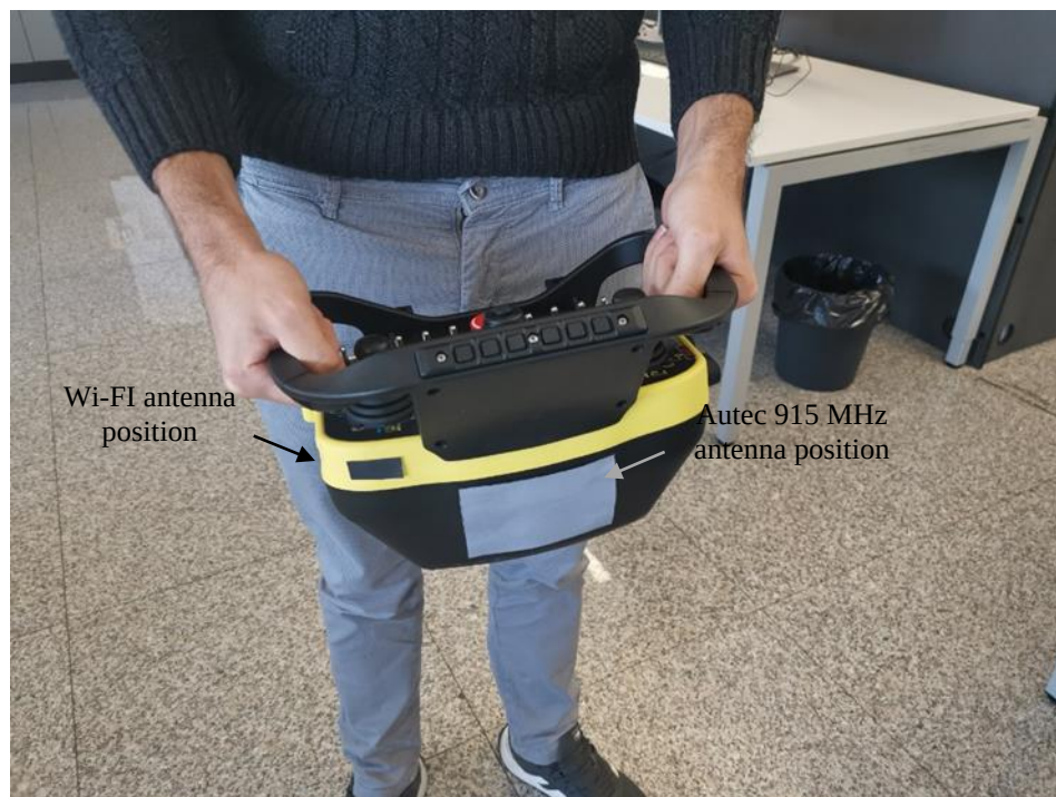
Figure F.6: Correct working position using PJM unit, front view
